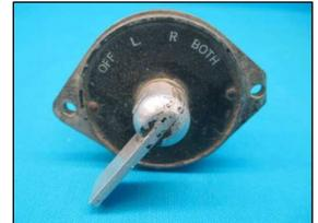
The AC-8 was used on L-5's to P-51's and any single engine aircraft of that period that used a 2-1/8" switch and carried a battery. You will now find many J-3's and L-4's, Aeronca L-3's, 7AC's, Taylorcraft and more with A-8 and A-9 switches).
