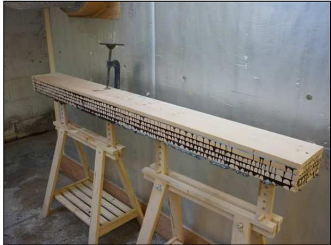
Beech planks laminated with Aerodux glue
