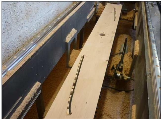
Urethane leading edge glued and cramped in prop blank
