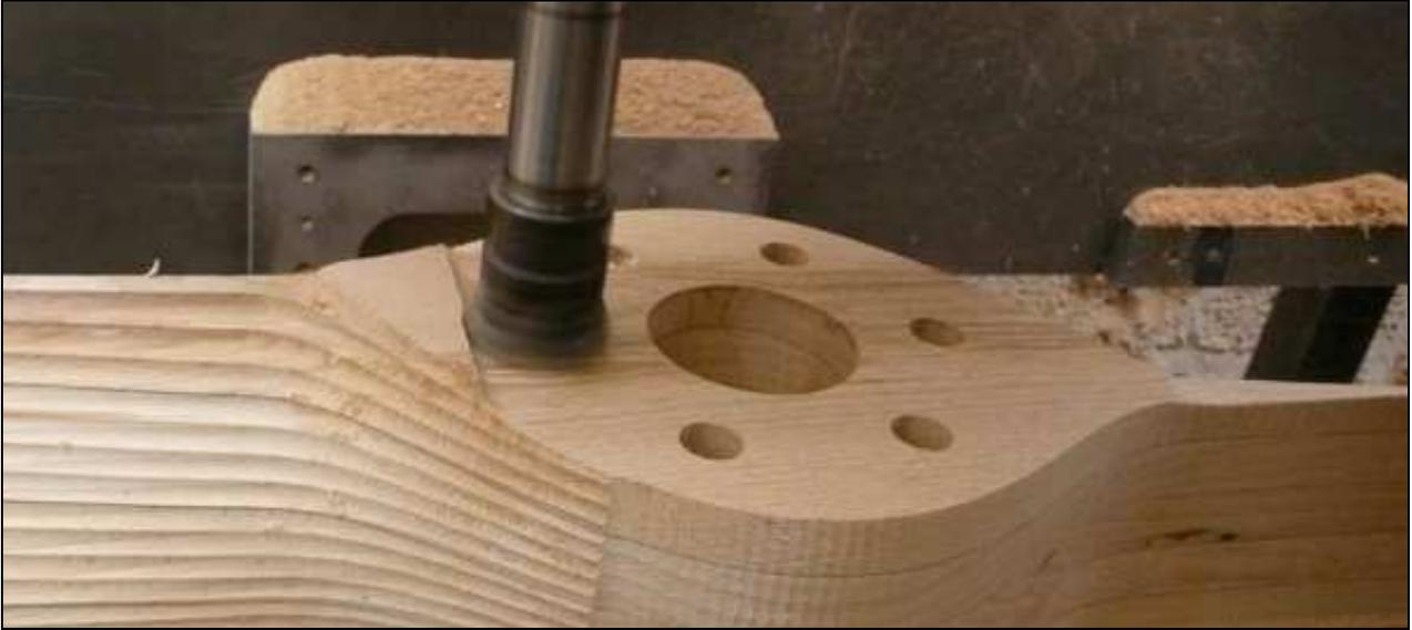
Router machine cutting prop profile (acknowledgements to Pilot magazine from the hercprop website)
