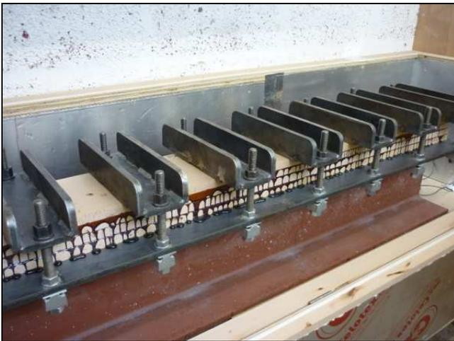
Glued blanks in clamping jig
