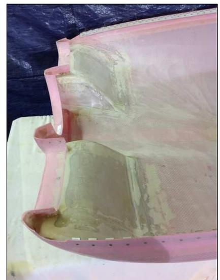
best part of two weeks, mainly due to the current temperatures and the curing time of the epoxy! The structure of the cowls is now all but complete with ducts, oil door and piano hinges in place, but, the real work of filling and priming is about to begin!!
