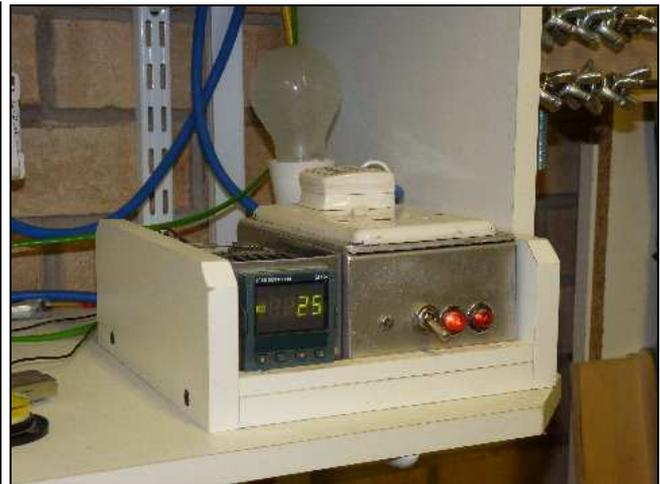
*Temperature control unit e.g. Eurotherm 2116 with home-made relay time-step regulator*
