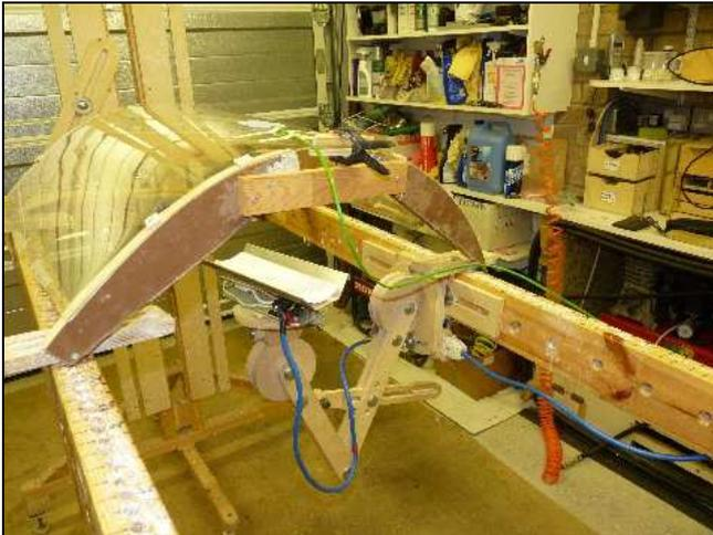
*IR heater in situ for annealing stage*
