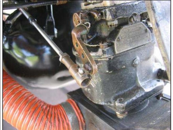
*Missing end screw but with trial fit of temporary spit pin*
