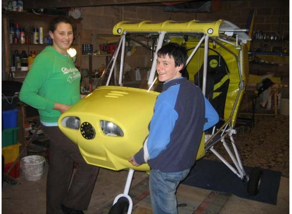
*Barnstaple crew. 31/01/08. Engine trial fitted and cowl clearance checked.*
